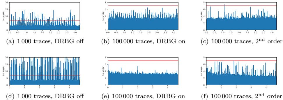
**Figure 6:** Results of TVLA assessment: the top row shows decompressed comparison for (a) 1<sup>st</sup> order without randomness, (b) 1<sup>st</sup> order with randomness, and (c) 2<sup>nd</sup> order with randomness, while the bottom row shows 1-bit compression for (d) 1<sup>st</sup> order without randomness, (e) 1<sup>st</sup> order with randomness, and (f) 2<sup>nd</sup> order with randomness. The  $x$  axis represents sample point index  $\times 10^6$ .
