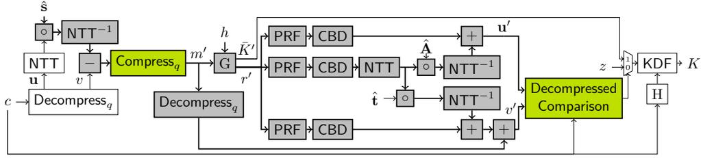
**Figure 1:** An overview of the various components in the Kyber CCA decapsulation. The components which need to be protected / masked are in color (gray or green) where we present new approaches for the green components.
